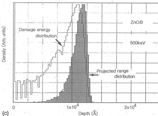
FIG. 3. Simulated depth profiles of implanted atoms with damaged layers of ZnO. (a)–(c) are for Ga at 2000 keV, Al at 1000 keV, and B at 500 keV, respectively.
