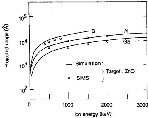
FIG. 4. Comparison of the projected range vs the ion energy obtained by simulation and experiment.
