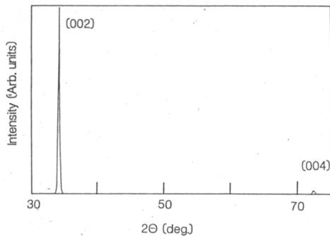
FIG. 1. X-ray diffraction pattern with a Cu K  $\alpha$  x-ray of the film of ZnO:Ga ( $1 \times 10^{17}$  ions/cm<sup>2</sup>) annealed at 400 °C for 4 h in N<sub>2</sub>.
