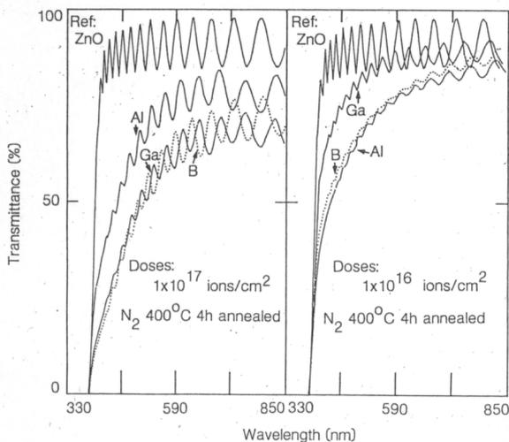
FIG. 2. Optical spectra in ultraviolet and visible region of the doped and nondoped ZnO films.
