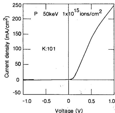
FIG. 1. Dark current-voltage characteristic of the homojunction diode of the P doped chalcopyrite structure Cu-In-Se thin film. The rectification ratio: K.
