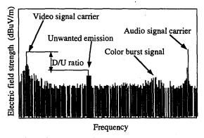
Fig. 2 Spectrum model of TV signal and unwanted emission.
