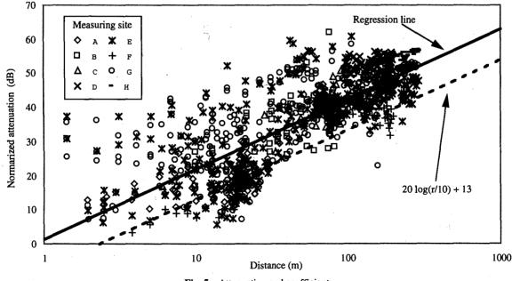
Fig. 5 Attenuation and coefficient.
