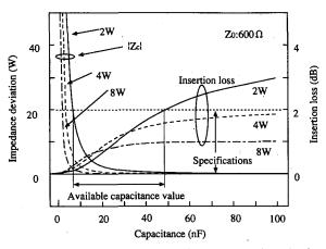
(a) Absolute value of common-mode impedance vs. insertion loss
