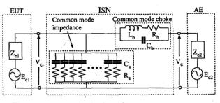
Fig. 6 Equivalent circuit of ISN for common mode current.
