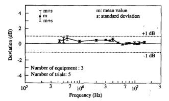
Fig. 15 Measurement deviation between two types of four-wire ISN.
