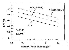
Fig. 10 Calculated result of longitudinal conversion loss.
