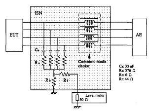
Fig. 13 Configuration of four-wire ISN.
