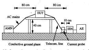
**Fig. 14** Layout for measuring disturbances at telecommunication ports.
