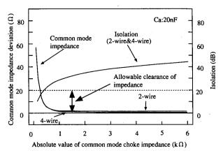
Fig. 9 Relation between common mode impedance and impedance of common mod choke.
