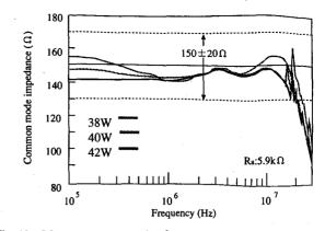
Fig. 12 Measurement example of common mode impedance of multiple-pair ISN.
