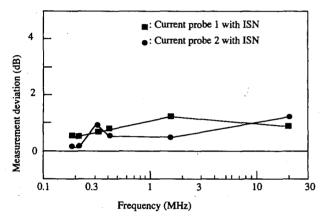
Fig. 16 Deviation in measurement results using current probes with ISN and using ISN alone.
