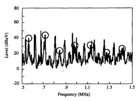
Fig. 3 Disturbance voltage measured by two 2W ISN.
