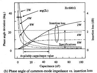
**Fig. 8** Relation between capacitance (Ca) and common mode impedance, and relation between insertion loss and common mode impedance. impedance and the design object of insertion loss for 2-wire balanced line, and Ca of about 20 nF is obtained for optimum value. These figure shows that the upper limit of the Ca value when number of wires is more than 4-wire.
