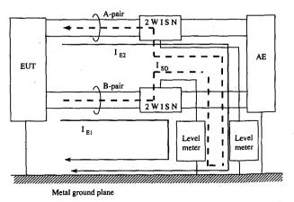
**Fig. 2** Equivalent circuit when two 2W ISN are used to measure disturbance voltage at telecommunication ports with 4W cable.
