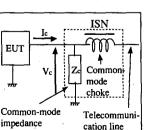
(b) Basic configuration of ISN Fig. 1 Basic concept and configuration of ISN.
