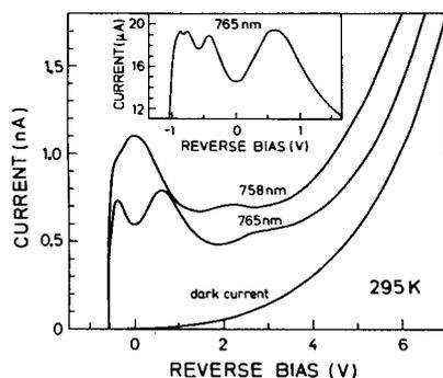
FIG. 2. Current vs reverse bias in the dark as well as for 758 and 765 nm illumination of a few nW. The inset corresponds to 300 mW illumination at 765 nm.
