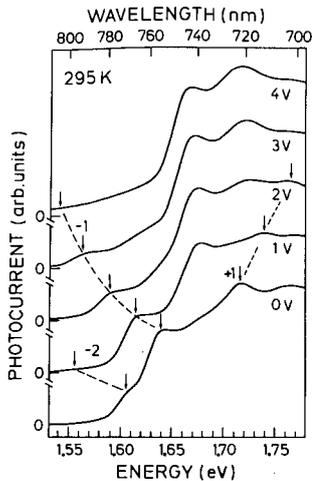
FIG. 1. Photocurrent spectra at different external reverse bias. The  $n = +1$ ,  $n = -1$ , and  $n = -2$  heavy-hole transitions are indicated by arrows.
