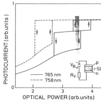
FIG. 3. Photocurrent vs illumination power ( $100 \mu\text{W}$  range) for 758 and 765 nm illumination at room temperature. The switching is indicated schematically; the arrows refer to its direction. The experimental circuit is displayed in the inset ( $V_B = 6$  V,  $R_V = 1$  M $\Omega$ ). The shaded area marks the region of switching between three stable states at 765 nm.
