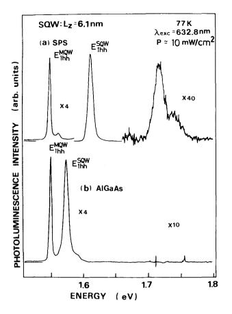
FIG. 1. 77 K photoluminescence spectra of two types of SQWH samples with (a) GaAs/AlAs SPS's and (b)  $Al_{0.24}Ga_{0.76}As$  cladding layers both with MQW buffer.
