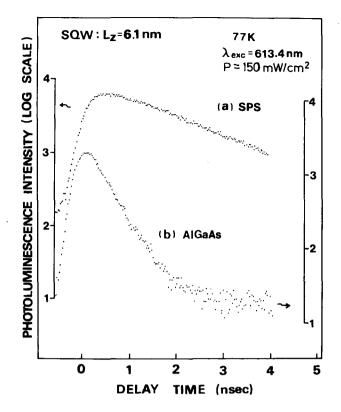
FIG. 2. Decay of the SQW photoluminescence intensity for two types of SQWH samples with (a) GaAs/AlAs SPS's and (b)  $Al_{0.24}$  Ga<sub>0.76</sub> As cladding layers both with MQW buffer.
