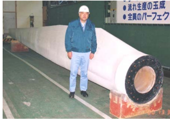
Fig.7.13 250kW Wind turbines and GFRP blades (Length: 12m)
