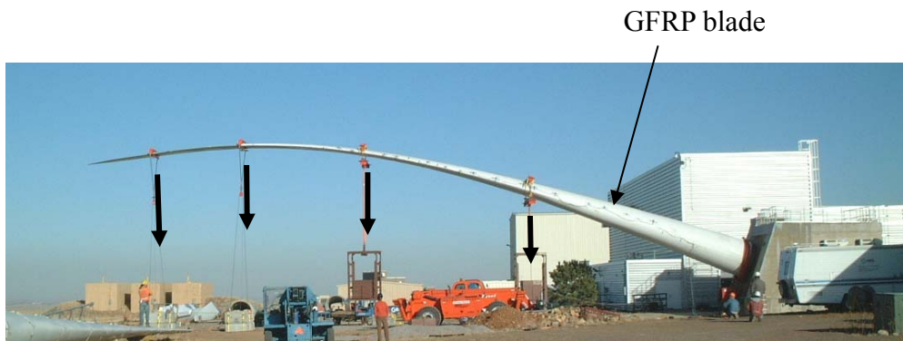
Fig.7.17 Static load test of GFRP blade
