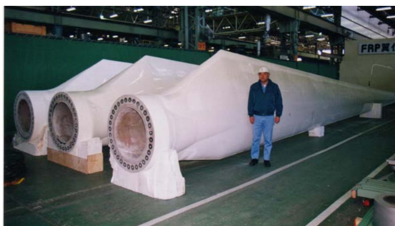
Fig.1.2 GFRP blades for 600kW Wind turbines (Length: 20m)
