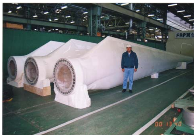
Fig.7.14 600kW Wind turbines and GFRP blades (Length: 18m)
