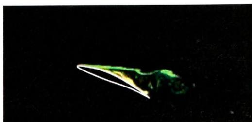
Fig. 3.3.8 Flow patterns around the stationary airfoil at  $\alpha = 16^\circ$
