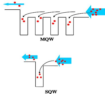
**Fig. 4** Schematic conduction band diagrams for carrier capturing by SQW and MQW structures (without including the internal field).
