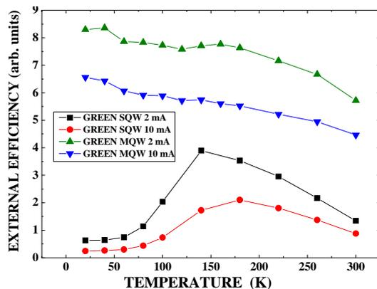
**Fig. 3** Temperature dependence of the integrated EL intensity for the green SQW and MQW diodes at two injection currents of 2 and 10 mA
