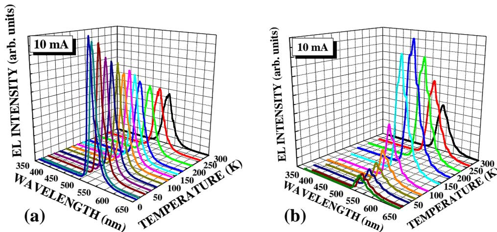
**Fig. 2** Temperature dependence of EL spectra for (a) green InGaN MQW-LED in comparison with (b) green SQW diode at a fixed injection current of 10 mA.
