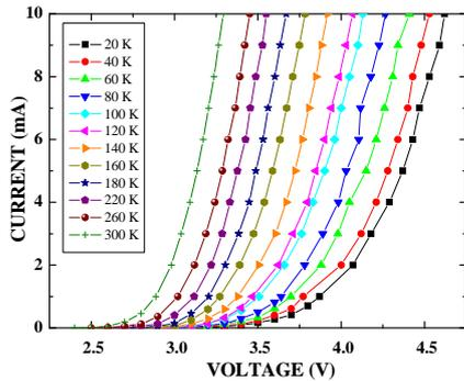
**Fig. 1** Current-voltage characteristics of the green InGaN MQW diode as a function of temperature between 20 and 300 K.
