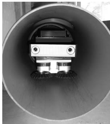
Fig. 3. The prototype autonomous sewer robot, KANTARO.
