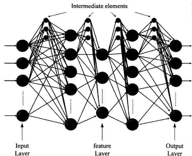
Fig. 2. A bottleneck neural network with intermediate elements in autoassociation
