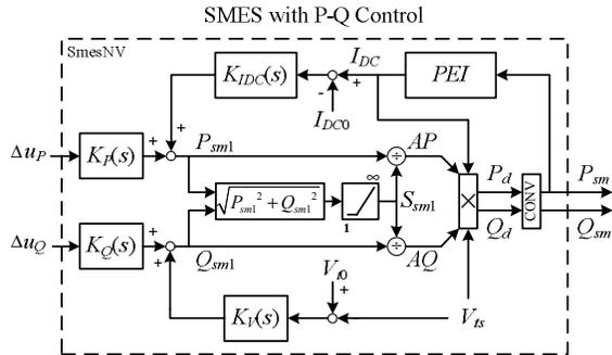
Fig. 1. SMES with P-Q controllers.
