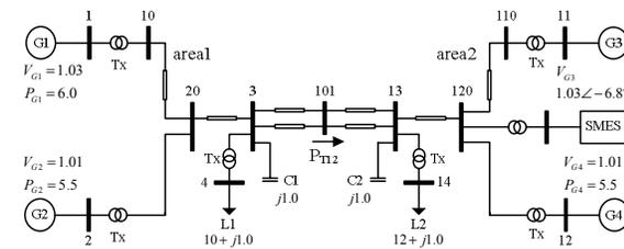
Fig. 6. Two area four machine power system.
