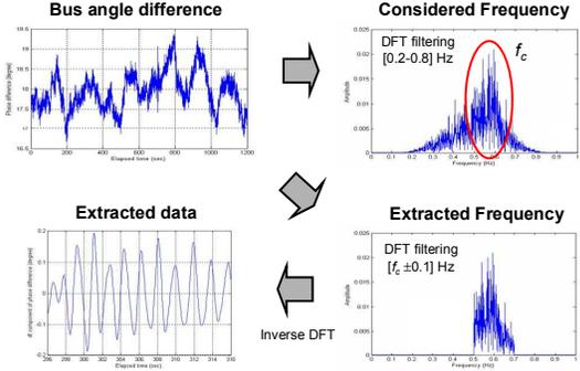
Fig. 4. Extraction of considered frequency component via DFT filtering.
