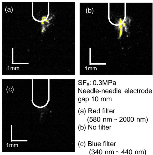
Fig.10. Spatial resolved PD light emission images with different wave filters in  $\text{SF}_6$  gas
