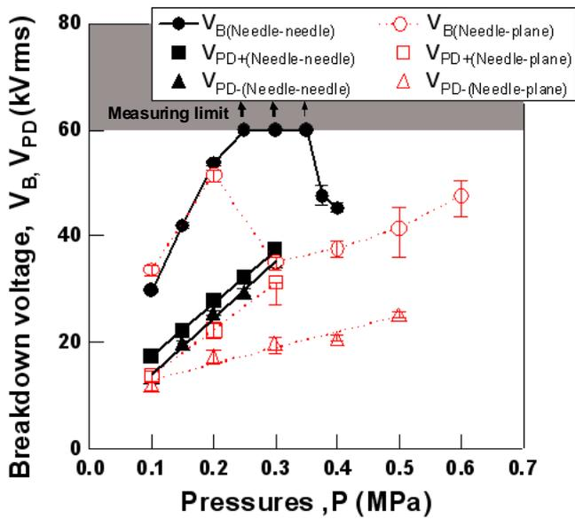
Fig.5. Gas pressure dependence of  $V_B$  and  $V_{PD}$  in  $SF_6$  gas
