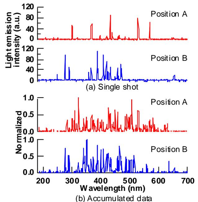
Fig.7. PD light emission spectra in  $SF_6$  gas at 0.3 MPa
