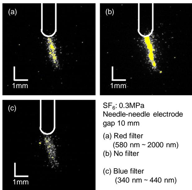
Fig.9. Spatial resolved PD light emission images with different wave filters in  $\text{SF}_6$  gas
