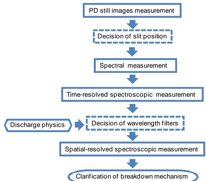
Fig.1. Flowchart of time and spatial-resolved spectrometric measurement
