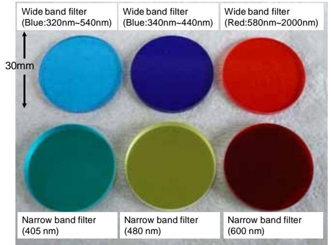
Fig.4. Photograph of the filters
