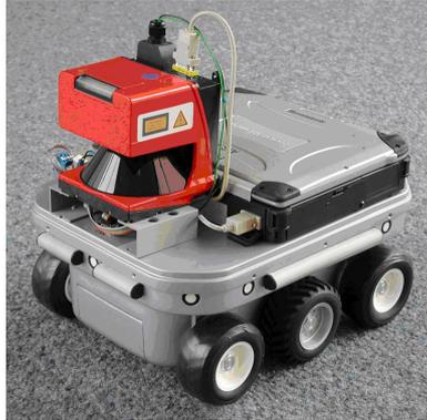
Figure 2.4: The commercial research robot platform, KURT2.
