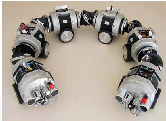
Figure 2.5: Automated inspection platform, MAKRO.
