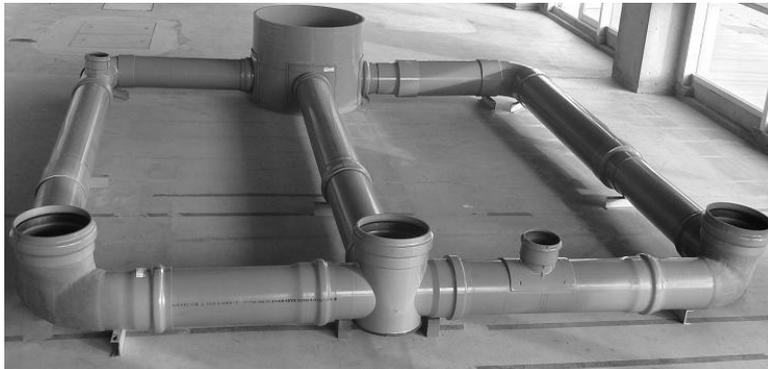
Figure 4.9: Dry sewer test field at the FAIS-RDSO.
