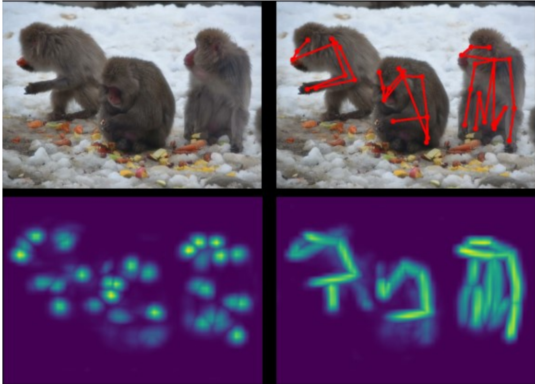
Figure 5.2: Visualization of the pose estimation process for a monkey. The input image (top left) is processed to generate the score map prediction (bottom left) and the PAF prediction (bottom right). The final output (top right) shows the detected key points and skeletal structure overlaid on the input image.
