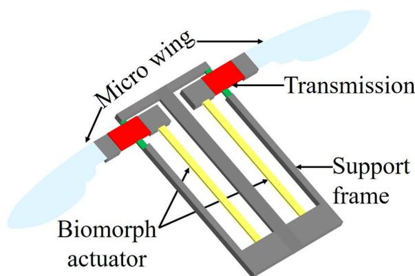
Figure 1: Concept of polymer micromachined flapping wing nano air vehicle or MEMS flyer.
