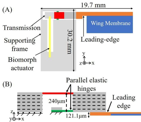
Figure 2: Actual design of FWNAV in plan (A) and section views (B). Note: Figures are the best views in color prints.
