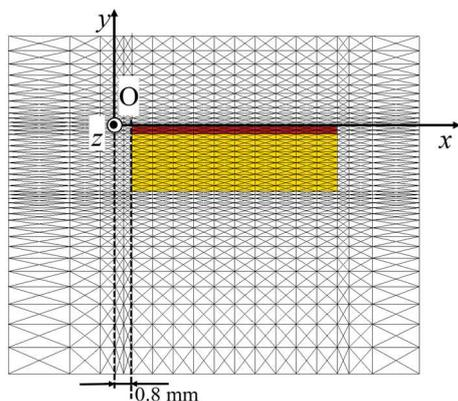
Figure 8: Applied fluid and wing mesh during FSI analysis.
