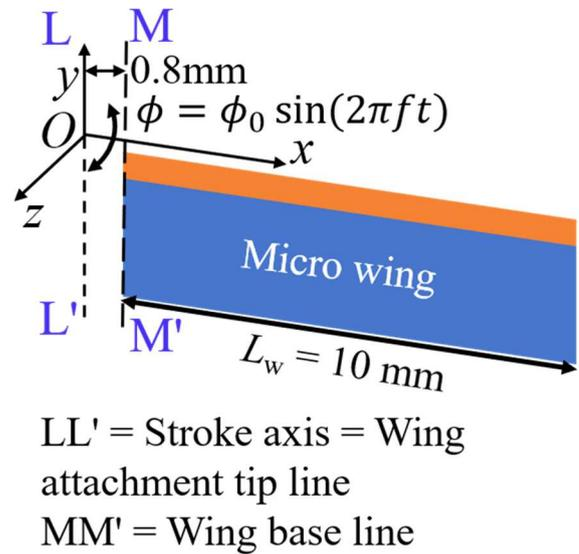
Figure 6: Problem setup for the fluid-structure interaction analysis of FWNAV.
