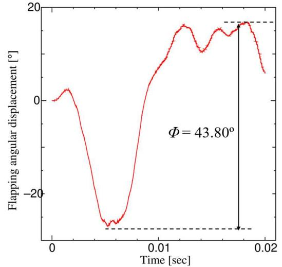
Figure 5: Time history of flapping angular displacement.
