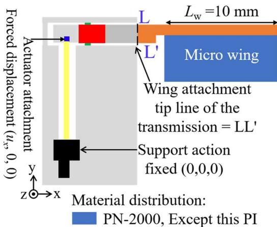
Figure 4: Problem setup for nonlinear structural dynamic analysis of FWNAV.
