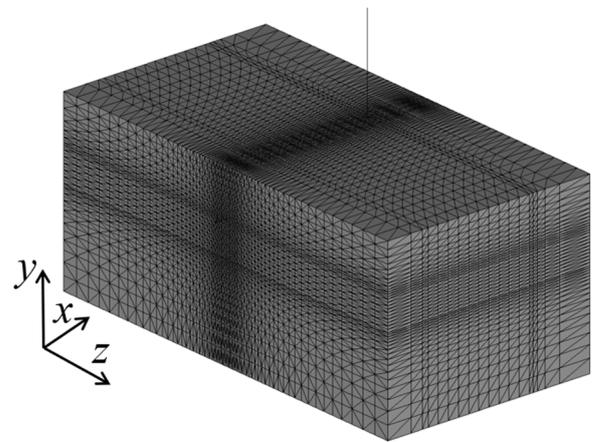
Figure 7: 3-D view of applied fluid mesh during FSI analysis.
