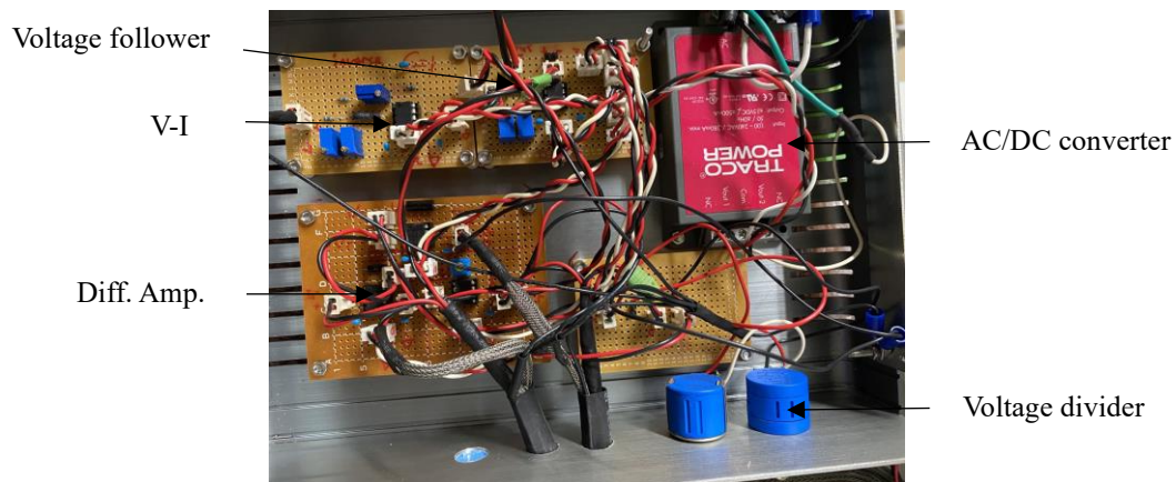
Fig. 2.22 Experimental circuit made according to the schematic.
