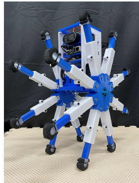
Fig. 12 Rimless wheel robot with elastic telescopic-legs
