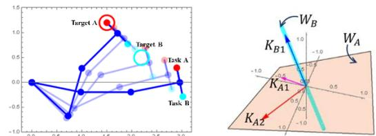
(a) Operation up to the target point A (b) Joint Space R3 (Target A)
