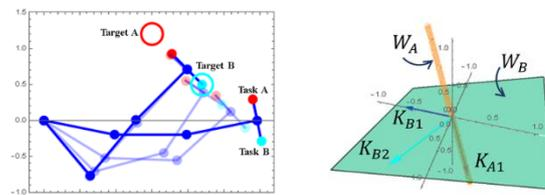
(a) Operation up to the target point B (b) Joint Space R3 (Target B)
