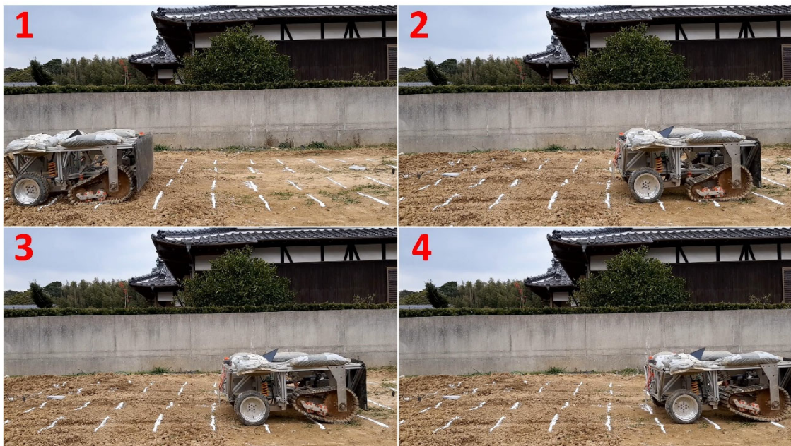
Figure 4-8 Experiment switch from track to wheel mode
