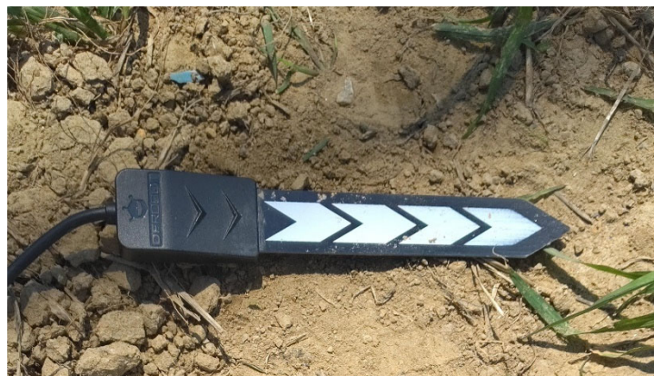
Figure 2-28 Analog Waterproof Capacitive Soil Moisture Sensor (SEN0308 DFRobot)
