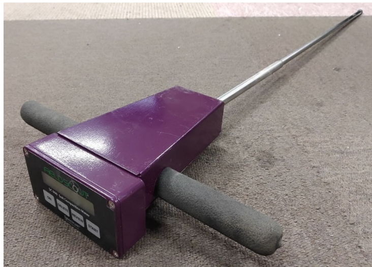
Figure 3-9 The digital cone penetrometer SC900
