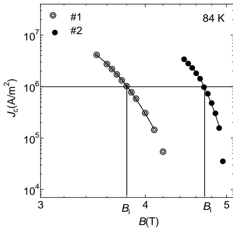
Fig.3 Enlarged figure for determination of irreversibility field.
