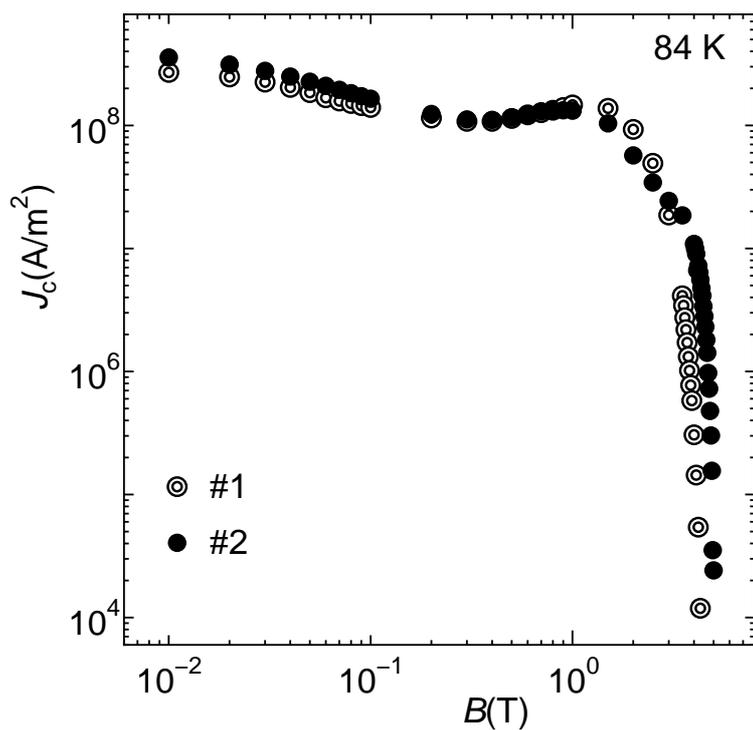
Fig.2 Magnetic field dependence of the critical current density of NEG-123 bulk oxide superconductors with different NEG-211 contents.
