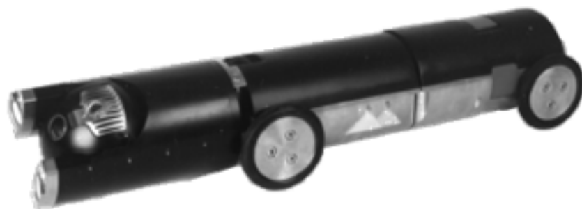
Figure 5.4: KARO is an experimental semi-autonomous carrier for sewer inspection sensory equipment. It was developed by a group of research institutes and some industrial partners in Germany.
