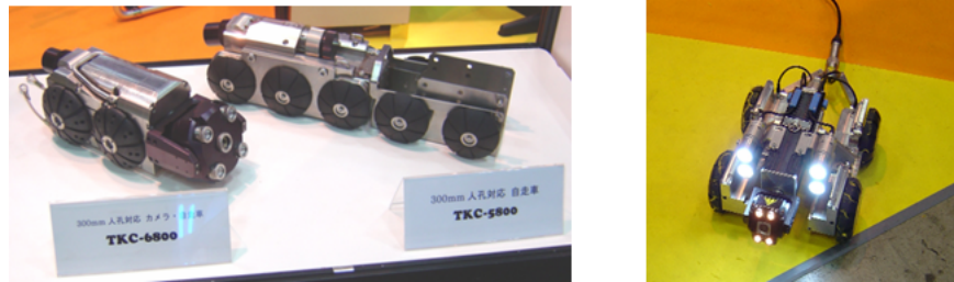
Figure 5.23: Three samples of current commercial sewer inspection robots (Q.I company - Japan).
