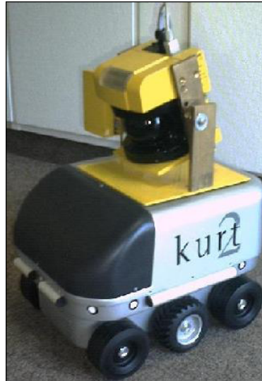
Figure 5.2: The commercial research robot platform KURT2. Figure shows a KURT2 system with a custom mounted 2D laser distance scanner.
