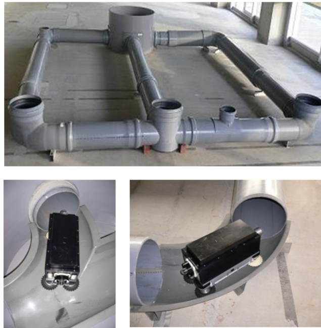
Figure 5.48: Our sewer test field including all kind of pipe bends at RRI laboratory. Two down pictures showed KANTARO when passing a junctions (Left side) and a 90 degree curve (Right side).
