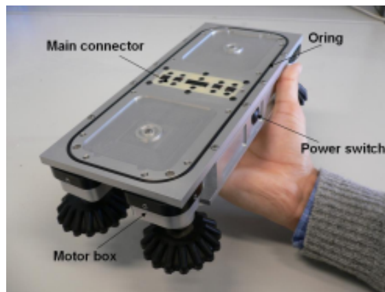
Figure 5.37: naSIR platform consists of naSIR mechanism, a lithium polymer battery pack fitted under the platform (is not show in the figure) and a power switch.
