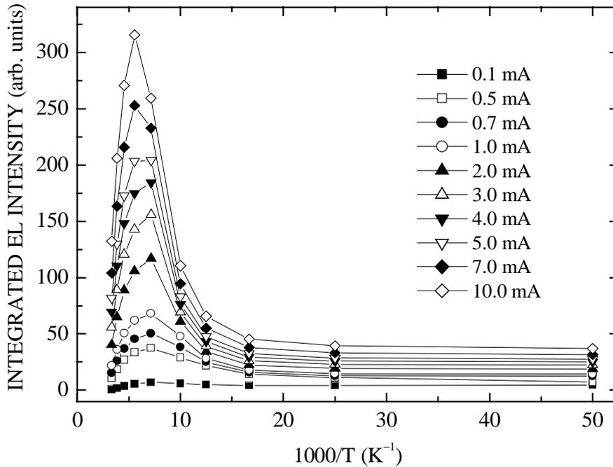
**Figure 2.** Spectrally integrated EL intensity of the green InGaN SQW LED as a function of inverse temperature at various injection currents from 0.1 to 10 mA.
