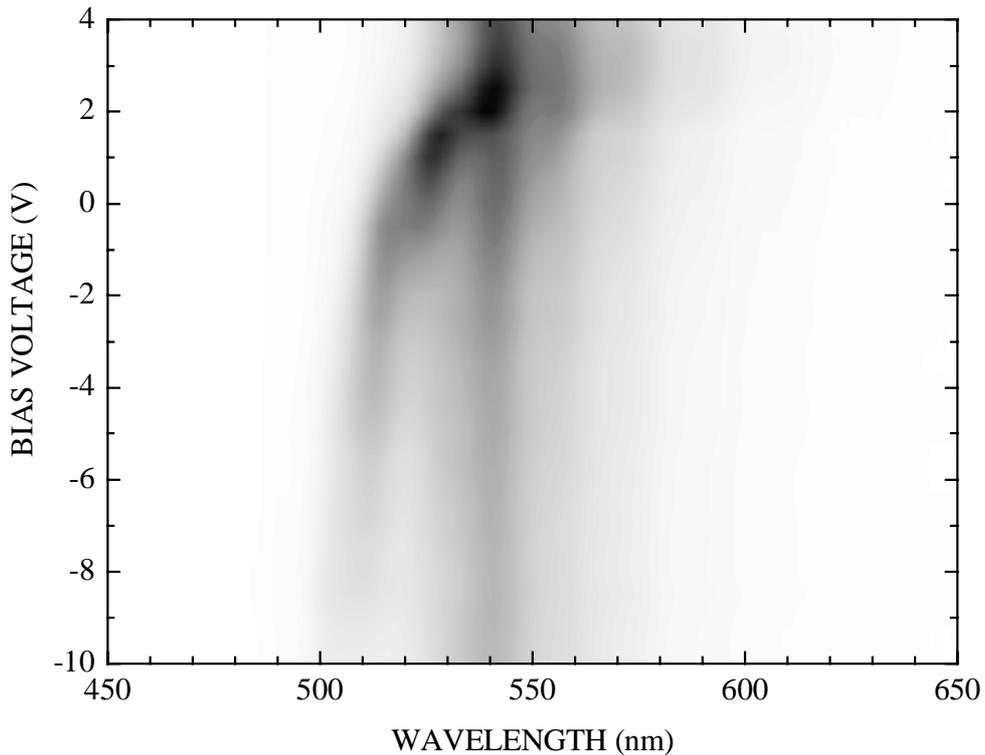
**Figure 3.** A grey-scale plot of PL spectral intensity of the green InGaN SQW LED as a function of wavelength and applied bias voltage measured at 15 K.
