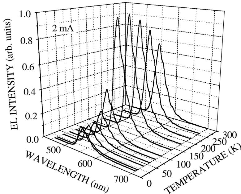
**Figure 1.** Temperature dependence of EL spectra of the green InGaN SQW LED at an injection current of 2 mA.
