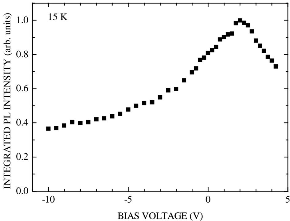
**Figure 5.** Spectrally integrated PL intensity of the green InGaN SQW LED at various applied bias voltages between  $-10$  and  $4.25$  V measured at  $15$  K.
