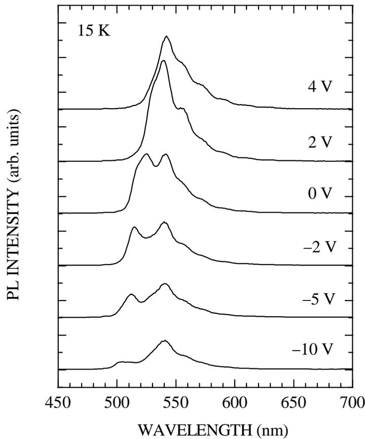
**Figure 4.** PL spectra of the green InGaN SQW LED measured at 15 K under applied bias voltages of  $-10$ ,  $-5$ ,  $-2$ ,  $0$ ,  $2$  and  $4$  V. Base lines of the PL spectra are vertically shifted for clarity.
