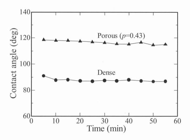
Fig.4 Change in contact angle as a function of measuring time for two-types of  $MnAl_2O_4$  spinel substrates measured at 1573K.
