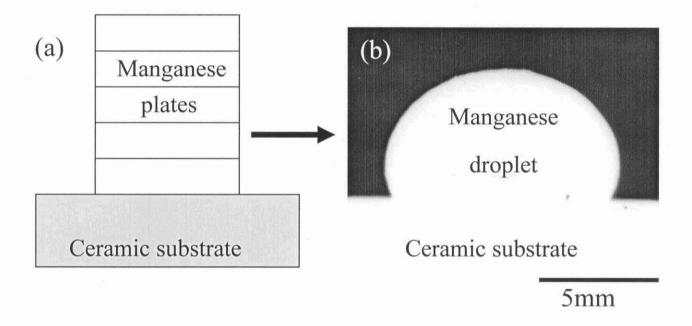
Fig.3 Manganese on substrate: a, manganese plates piled up on substrate before heating; b, photograph of manganese droplet immediately after melting.
