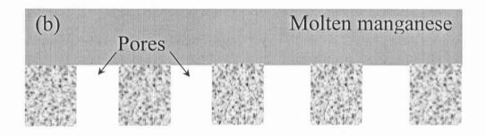
Fig.7 Simplification of porous interface in order to estimate apparent contact angle on the basis of Cassie and Baxter's equation<sup>[7]</sup>: a, molten manganese-porous substrate interface; b, simplified model for porous interface.
