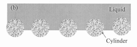
Fig.6 Two interfacial models: a, Wenzel's model for rough surface<sup>[6]</sup>; b, Cassie and Baxter's model for porous surface<sup>[7]</sup>.
