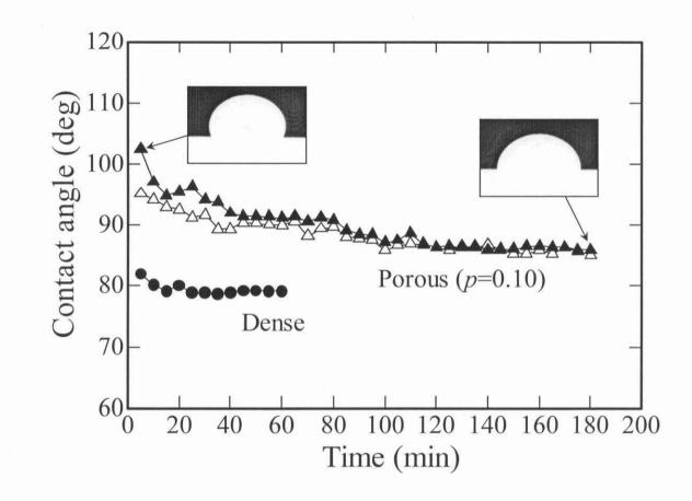
Fig.5 Change in contact angle as a function of measuring time for two-types of  $ZrO_2$ -4.6mass% $Y_2O_3$ -9.9mass%MnO substrates measured at 1573K.
