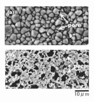
Fig.1 SE images of surfaces of  $\rm MnAl_2O_4$  spinel substrates: a, dense substrate produced by manganese-alumina heated for one hour at 1773 K; b, porous substrate sintered at 1673 K for 2 hrs.
