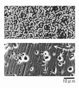
Fig.2 SE images of surfaces of  $\rm ZrO_2$ -4.6mass% $\rm Y_2O_3$ -9.9mass%MnO substrates: a, dense substrate produced by manganese-zirconia(yttria) heated for one hour at 1773 K; b, porous substrate sintered at 1673 K for 2 hrs.
