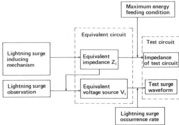
Fig. 2. Design flow for the lightning surge test circuit and the test waveform.
