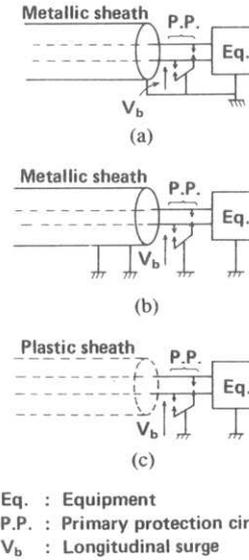
Fig. 7. Standard connecting configuration between the equipment and the telecommunication line. (a) Cable metallic sheath is connected to the equipment ground and P.P. ground. (b) Cable metallic sheath ground, equipment ground, and P.P. ground are separated. (c) Cable has no metallic sheath.
