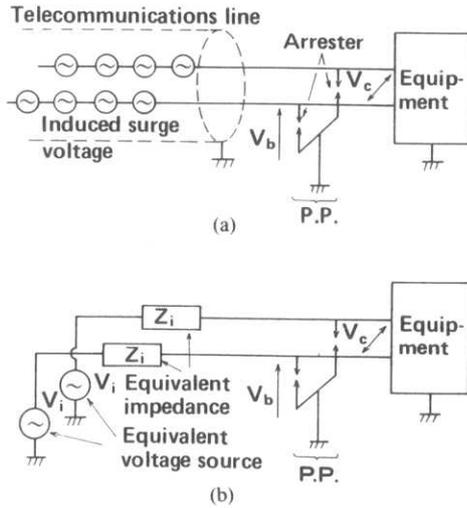
Fig. 1. Lightning surge test circuit for equipment. (a) Telecommunication line within the distributed electromotive force-induced lightning surge, and the lightning surge fed to the equipment and its protection circuit. (b) Basic construction of the new test circuit.
