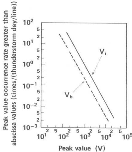
Fig. 9. Peak value occurrence rate greater than abscissa values of the observed surge  $V_b$  and the equivalent voltage source  $V_i$  at the subscriber end.
