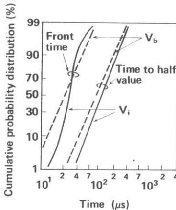
Fig. 10. Front time and time to half value distributions of the observed surge  $V_b$  and equivalent voltage source  $V_i$  at the subscriber end.
