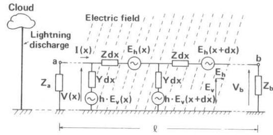
Fig. 3. Lightning surge induction model for the circuit between one wire of the balanced pair and ground.
