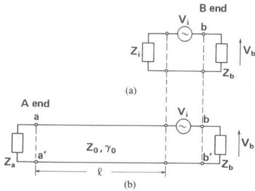
Fig. 4. Equivalent circuit for Fig. 3. (a) Lightning surge  $V_b$  at the telecommunication line end  $B$  is represented by the equivalent impedance  $Z_i$  and equivalent voltage source  $V_i$ . (b) Lightning surge  $V_b$  is represented by a transmission line and a equivalent voltage source  $V_i$ .
