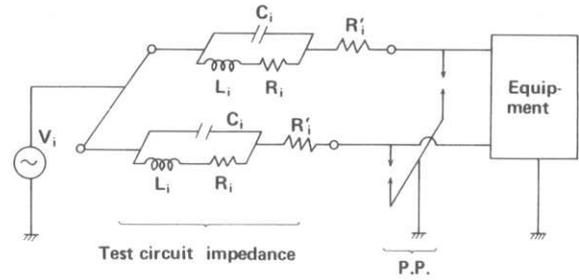
Fig. 6. New test circuit for the equipment at the subscriber end
