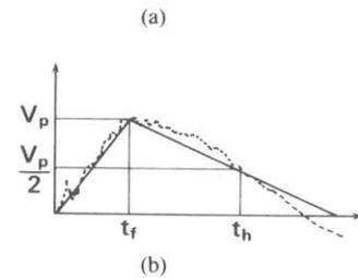
Fig. 5. Typical lightning surge waveform. (a) Lightning surge observed by the lightning surge waveform recorder. (b) Definition of the peak value, the front time, the time to half value and the triangular waveform.
