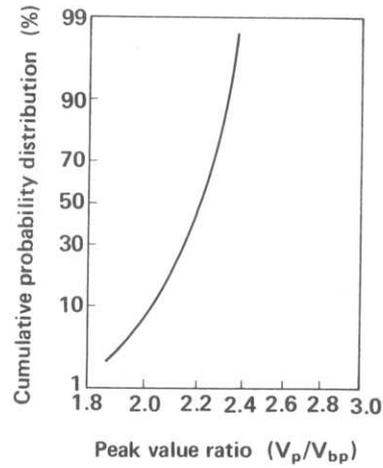
Fig. 12. Cumulative probability distributions of the peak value ratio ( $V_p/V_{bp}$ ).
