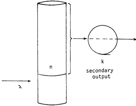
Fig. 3 Infinite queue model (M/M/∞)
