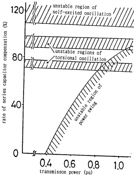
Figure 3. Result of calculating unstable regions for different amounts of transmission power.
