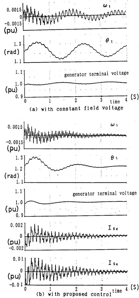
Figure 8. Simulated waveforms of the cases without control and with the proposed stabilizing system.
