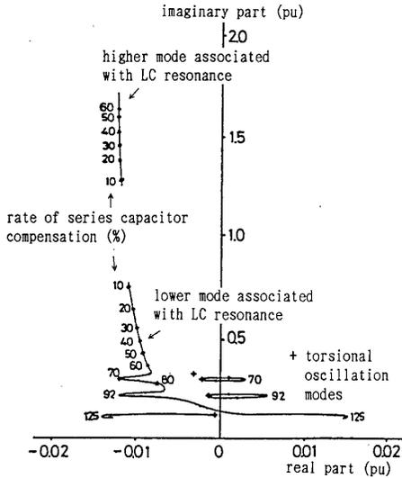
Figure 2. Result of calculating system eigenvalues associated with LC resonance for different series capacitor compensation rates.
