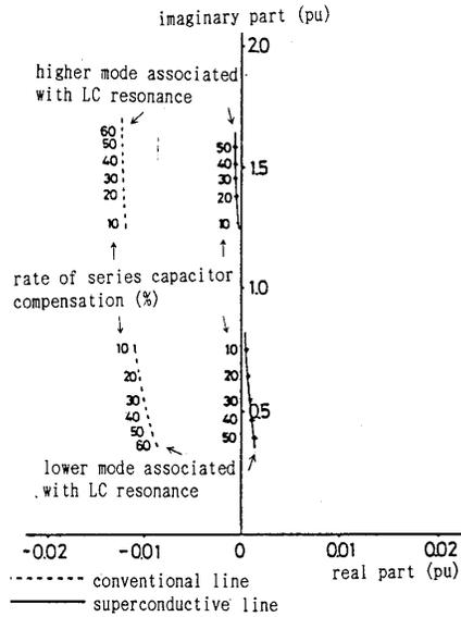
Figure 4. Result of calculating system eigenvalues associated with LC resonance in the model power system with superconductive power transmission line.
