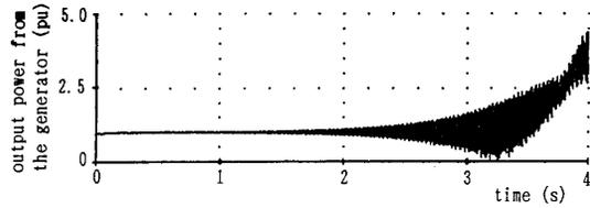
Figure 5. Simulated waveform in which self-excited oscillation is unstable.
