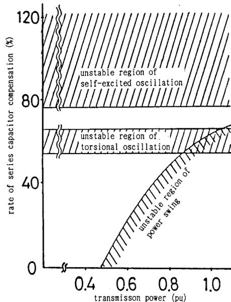
Figure 6. Results of calculating unstable regions in the power system with superconductive generator.
