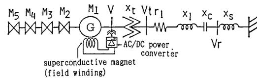
Figure 7. A configuration of the power system including superconductive generator with a power system stabilizing controller.
