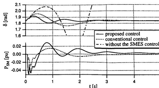
Fig. 9. Dynamic responses of the system at the heavy power flow case.
