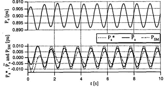
Fig. 6. Result of generator power control by the SMES.
