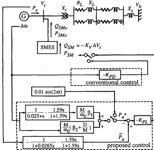
Fig. 5. Long distance bulk power transmission system with SMES.
