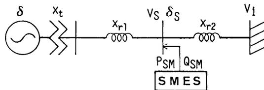
Fig.1. Long distance bulk power transmission system with SMES.
