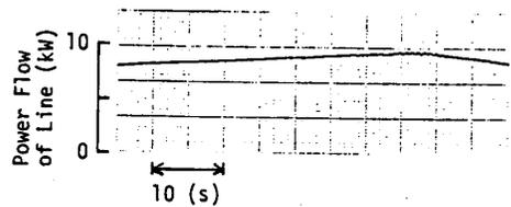
(b) with control using active and reactive power ( $K_D = 0.13$  [pu/(rad/s)],  $K_V = 3.4$  [pu/pu])
