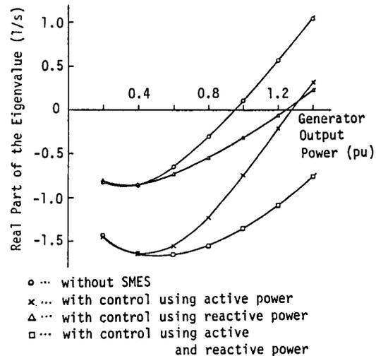
Fig.7. Variation of the real part of the eigenvalue for different generator outputs.
