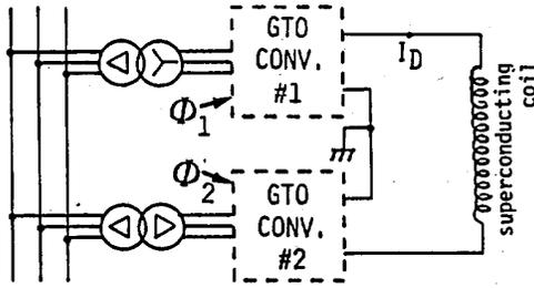
Fig.2. Fundamental configuration of a SMES.
