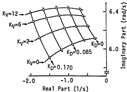
Fig.5. Variation of the eigenvalue with respect to control gains  $K_D$  and  $K_V$ .
