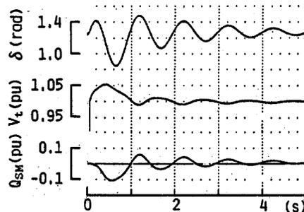
(b) with control using reactive power
