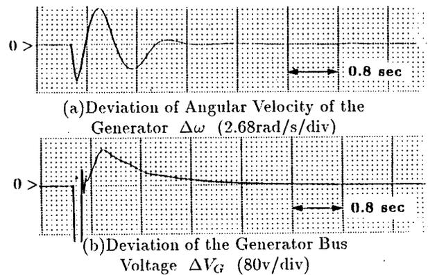
Fig. 5. With Control of the SuperSMES with Control Scheme 1)
