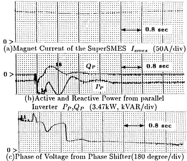
Fig. 7. With Control of the SuperSMES with Control Scheme 2)
