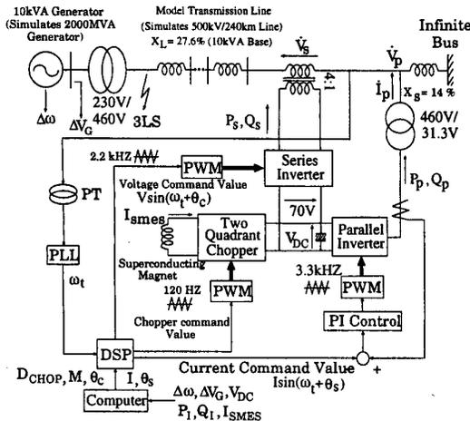
Fig. 2. Configuration of the Experimental System
