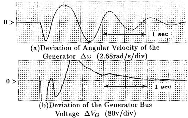
Fig. 4. With control of the SMES with Control Scheme 1)
