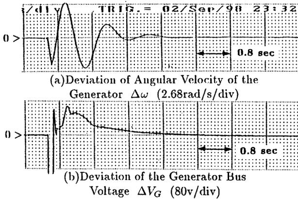
Fig. 6. With Control of the SuperSMES with Control Scheme 2)
