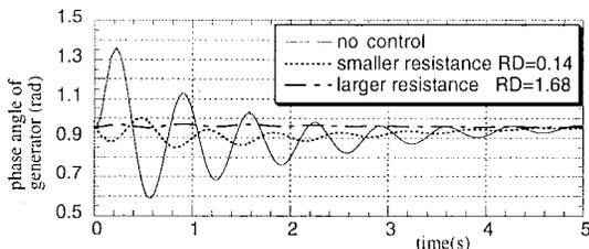
Fig. 4. Phase angle behavior of generator when a 3LG fault occurs near the generator.
