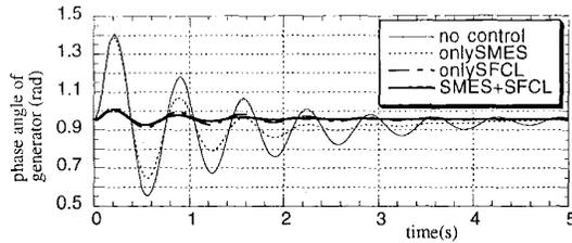
Fig. 7. Phase angle of generator when a 3-LG fault occurs at the point apart from the generator by 0.2 pu reactance. (The resistance of SFCL is 1.68pu).
