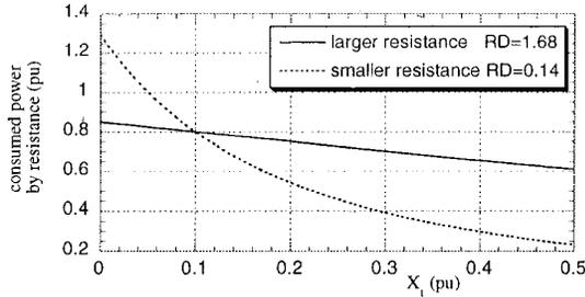
Fig. 2. Variation of consumed power by resistance for different amounts of reactance.
