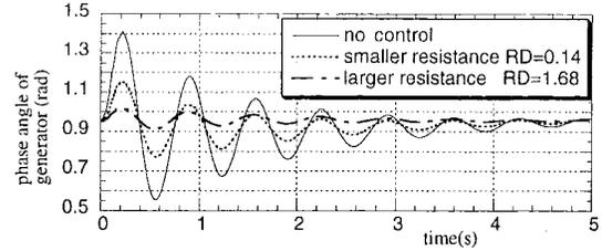
Fig. 5. Phase angle behavior of generator when a 3LG fault occurs at the point apart from the generator by 0.2 pu reactance.
