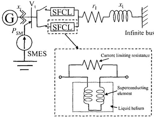
Fig. 1. Model power system with SMES and SFCL.
