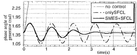
Fig. 8. Generator phase angle curve when the damping of power swing is weak.
