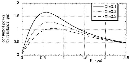
Fig. 3. Variation of consumed power by resistance for different values of resistance.
