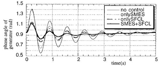
Fig. 6. Phase angle of generator when a 3-LG fault occurs at the point apart from the generator by 0.2 pu reactance. (The resistance of SFCL is 0.14pu).
