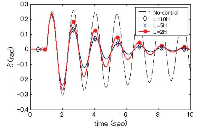
Fig. 4. Deterioration of SMES effective performance (Power angle  $\delta$ ).
