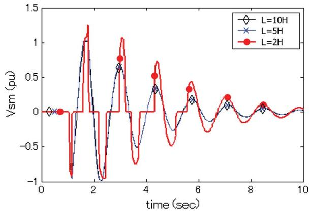
Fig. 5. SMES coil voltage  $V_{sm}$  due to stored energy capacity.
