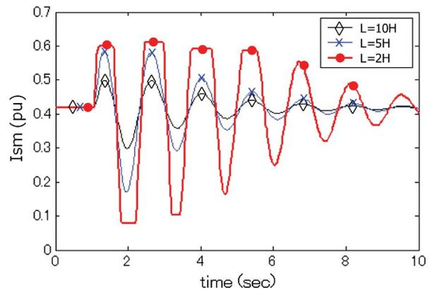
Fig. 7. SMES coil current  $I_{sm}$  due to stored energy capacity.
