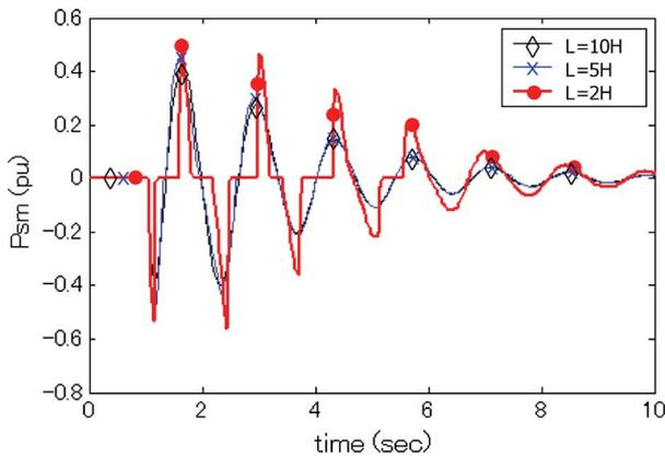
Fig. 6. SMES output  $P_{sm}$  due to stored energy capacity.
