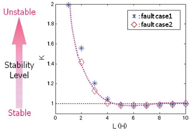
Fig. 3.  $L - K$  relationship for heavy load conditions.
