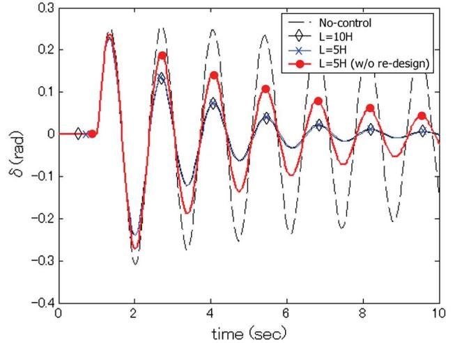
Fig. 2. Comparison of SMES effective performance (power angle  $\delta$ ).
