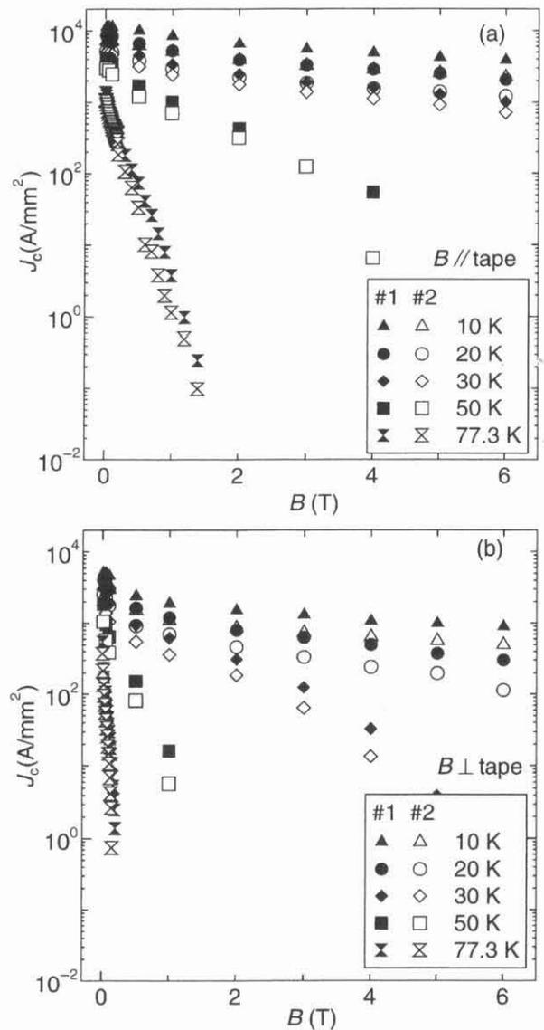
Fig. 7. Magnetization critical current density at various temperatures in magnetic fields (a) parallel to the tape and (b) normal to the tape.
