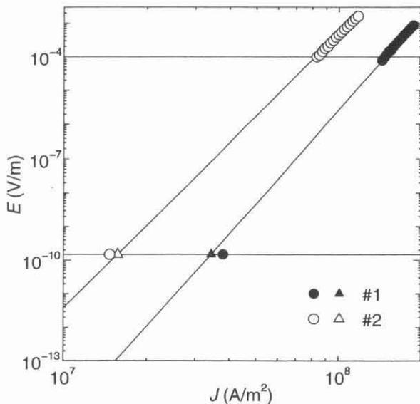
Fig. 6. Estimation of magnetization critical current density by extrapolating the  $E - J$  curve of resistive measurements. Triangular symbols show the estimated values. Observed magnetization critical current density is also shown for comparison.
