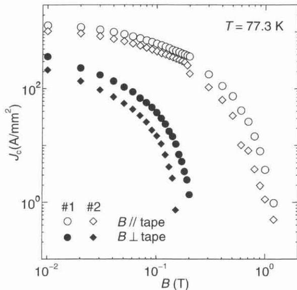
Fig. 5. Magnetic critical current density of specimens #1 and #2 in a magnetic field parallel and normal to the tape surface at 77.3 K.
