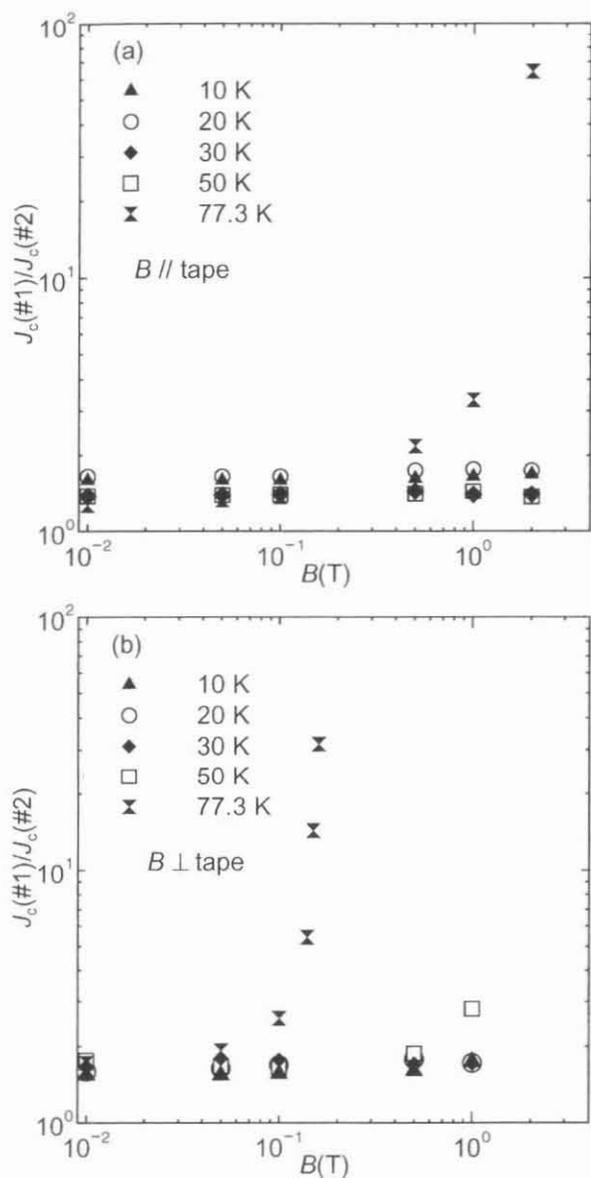
Fig. 8. Factor of improvement of magnetization critical current density by the over pressure processing for a magnetic field (a) parallel and (b) normal to the tape surface.
