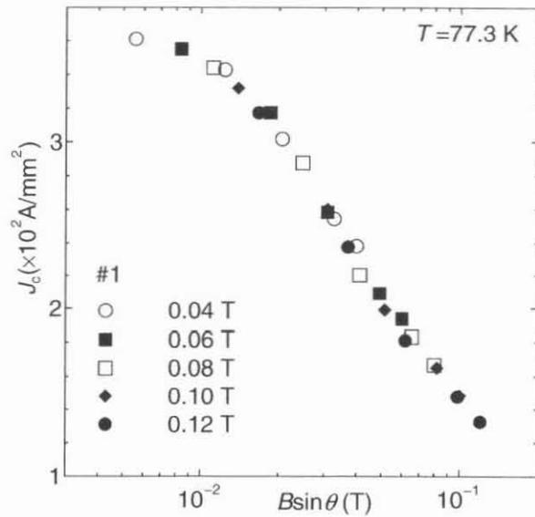
Fig. 3. Transport critical current density of specimen #1 versus a magnetic field component normal to the tape surface at 77.3 K.
