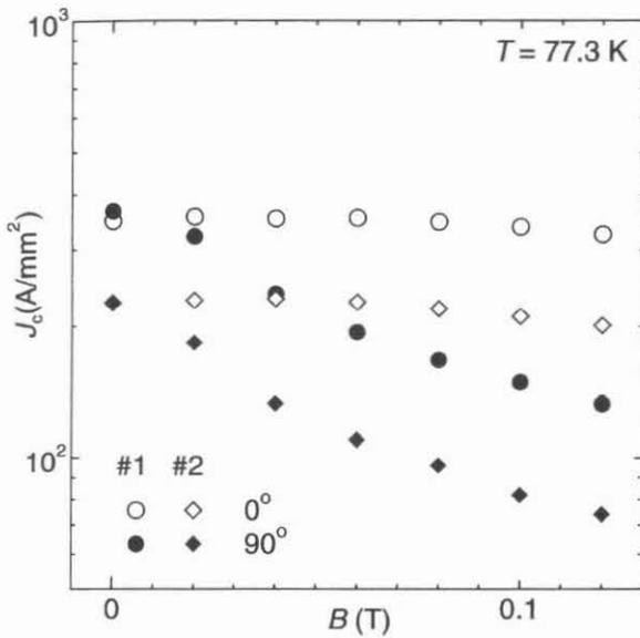
Fig. 1. Transport critical current density of specimens #1 and #2 in a magnetic field parallel and normal to the tape surface at 77.3 K.
