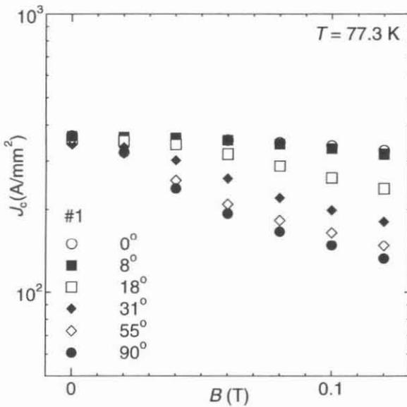
Fig. 2. Transport critical current density of specimen #1 in a magnetic field of various directions at 77.3 K.
