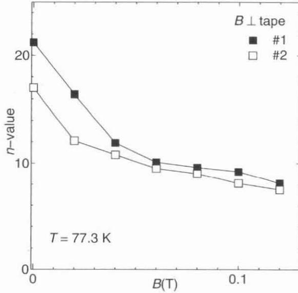
Fig. 4. *n* value of specimens #1 and #2 in a magnetic field normal to the tape surface.
