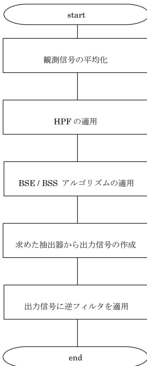
Fig. 5.8. The flow of the proposed algorithm.
