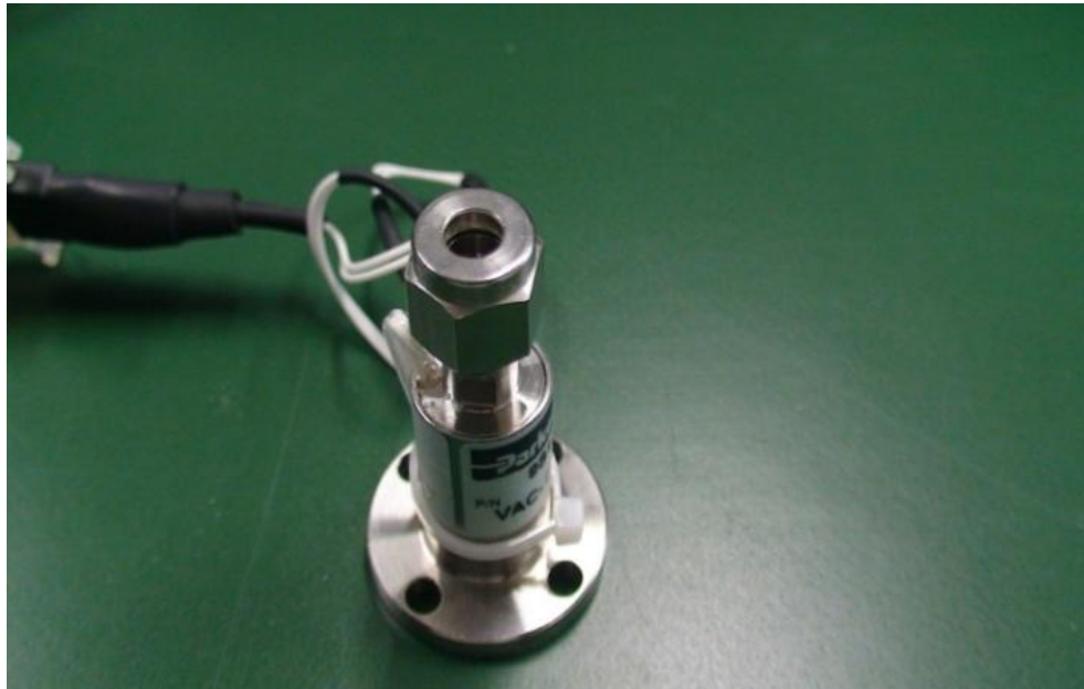
Figure 2.5: Pulse valve used for injecting molecular oxygen into nozzle.
