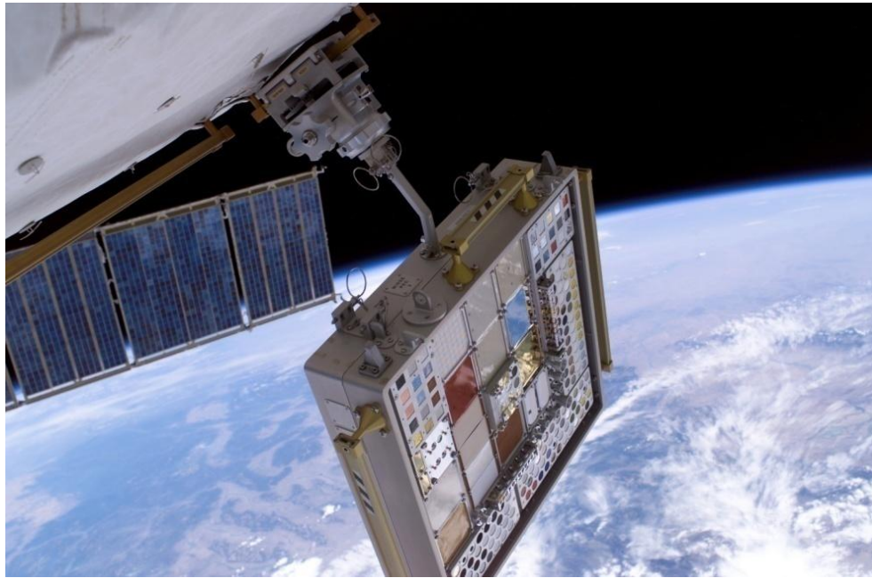
Figure 1.9: MISSE experiments being carried out at ISS in space
