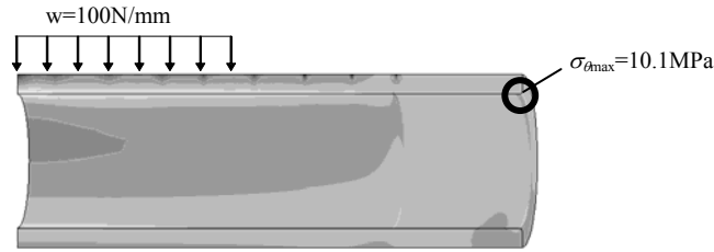
Fig. 4.5 Stress distribution \sigma_\theta when the sleeve and shaft are perfectly bonded as unit body
