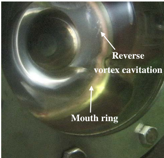
(2) Reverse vortex cavitation
