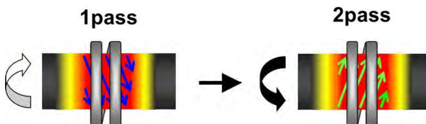
Fig.3.2.5 Image of multiple CREO treatment
