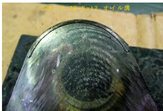
Fig.4.3.10 Outlook of products with lubricant pocket
