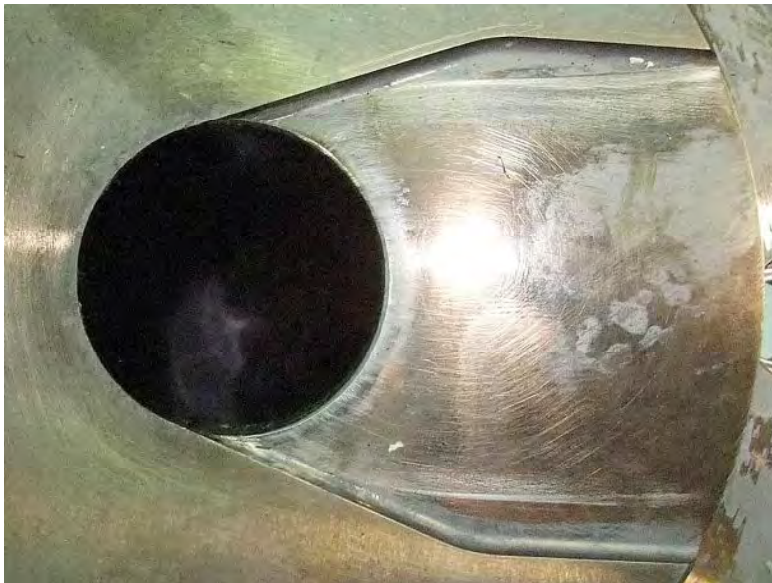
Fig.4.3.32 Outlook of lower die surface after forging
