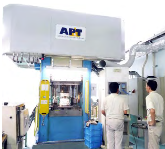
Fig.4.2.4 Photograph of hydraulic press with 4 cylinder
