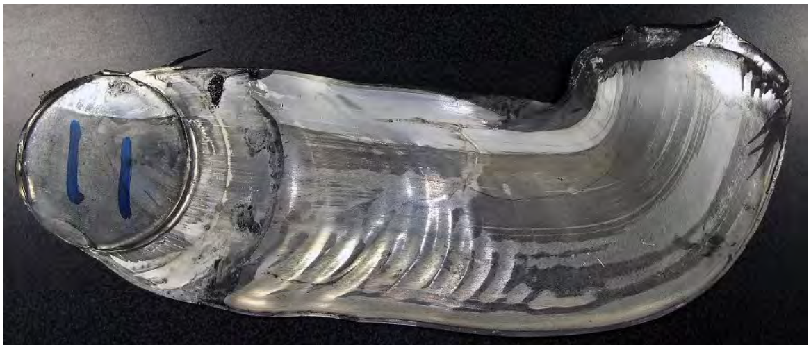
Fig.4.3.29 Outlook of short billet forging
