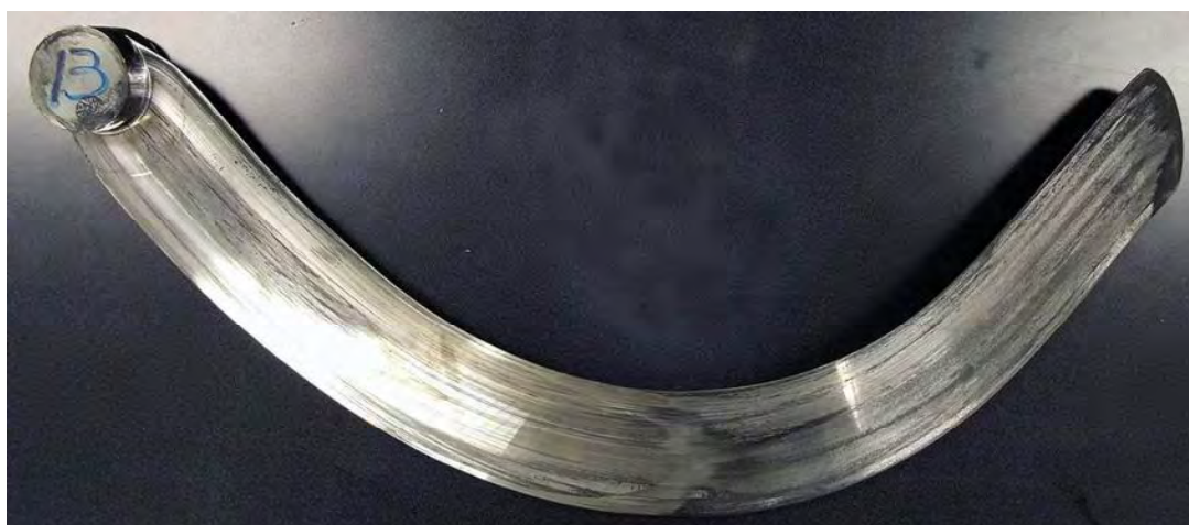
Fig.4.3.25 Outlook of lateral extrusion product from 2 direction
