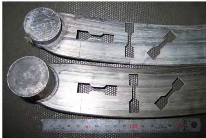
Fig.4.3.22 Position of tensile test specimens
