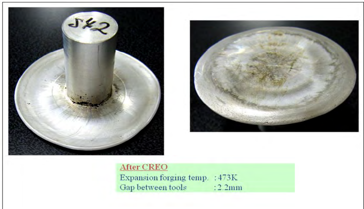
Fig.4.1.12 Outlook of expansion forging of CREO treated AZ61 at 200 with 2.2mm tool gap
