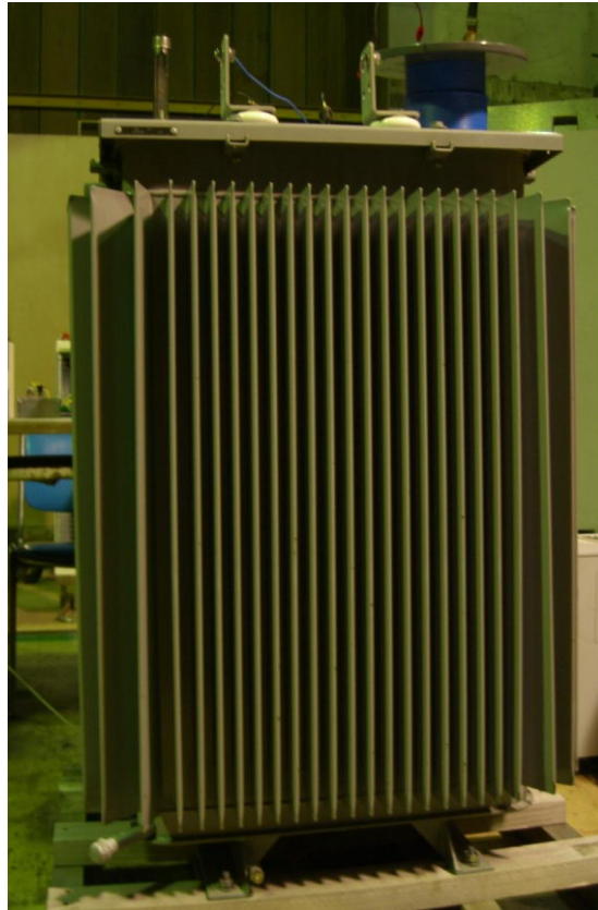
Fig. 4.13 Photograph of 300 kVA oil-immersed transformer (Hamakawazaki, Toshiba)
