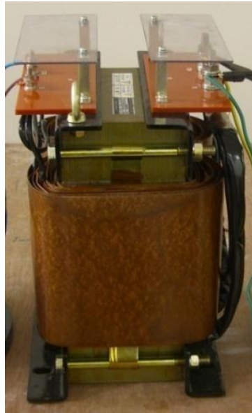
Fig. 3.11 The photograph of tested 4 kVA transformer
