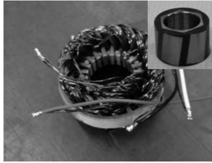
図 53 Internal motor construction
