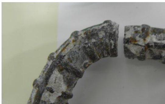
写真-4.5 case14・C 鉄筋 ( 0.75d )・破断鉄筋
