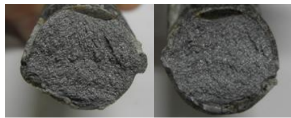
写真-4.6 case14・C 鉄筋 ( 0.75d ) 破断鉄筋
