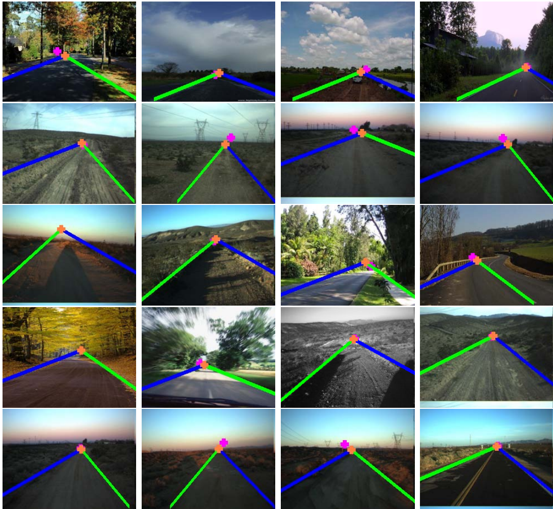
Figure 3.27: Examples of road area extraction for dark roads. Pink crosses: initial VPs, orange crosses: updated VPs, bright green lines: first detected borders, blue lines: second detected borders.
