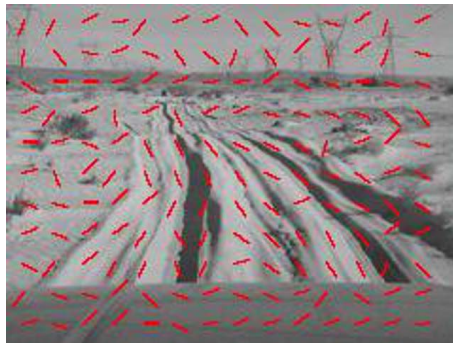
Figure 2.6: Sampled texture orientations (red segments) by Gabor filters.
