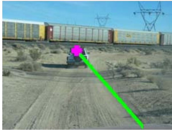
(b) First border detection: select an angle with maximum h(\text{angle}) in the histogram.
