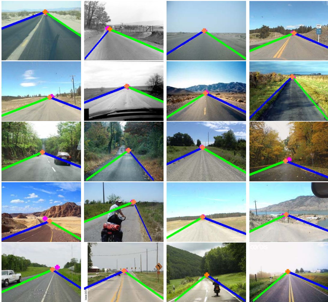
Figure 3.24: Examples of road area extraction for structured roads. Pink crosses: initial VPs, orange crosses: updated VPs, bright green lines: first detected borders, blue lines: second detected borders.
