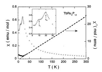
FIG. 3. Magnetic susceptibility  $\chi$  (open circles) at H=1 T and inverse magnetic susceptibility  $\chi^{-1}$  (filled circles) vs temperature for TbRu<sub>4</sub>P<sub>12</sub>. The line shows a fit to a Curie-Weiss law for 150 < T < 300 K. Inset: an enlarged view of  $\chi$  below 20 K.
