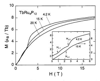
FIG. 5. Magnetization curves M(H) for TbRu<sub>4</sub>P<sub>12</sub> at several temperatures. Inset: magnetization curves at 4.2 K and 15 K below 6 T.
