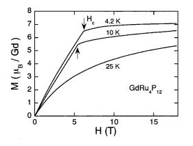
FIG. 4. Magnetization curves M(H) for GdRu<sub>4</sub>P<sub>12</sub> at several temperatures.
