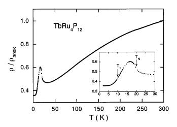
FIG. 7. Normalized electrical resistivity  $\rho/\rho_{300 \text{ K}}$  vs temperature for TbRu<sub>4</sub>P<sub>12</sub>. The inset shows an enlarged view below 30 K.
