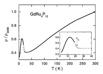
FIG. 6. Normalized electrical resistivity  $\rho/\rho_{300 \text{ K}}$  vs temperature for GdRu<sub>4</sub>P<sub>12</sub>. The inset shows an enlarged view below 40 K.
