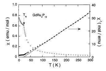
FIG. 2. Magnetic susceptibility  $\chi = M/H$  (open circles) at H = 1 T and inverse magnetic susceptibility  $\chi^{-1}$  (filled circles) vs temperature for GdRu<sub>4</sub>P<sub>12</sub>. The line shows a fit to a Curie-Weiss law for 150 < T < 300 K.
