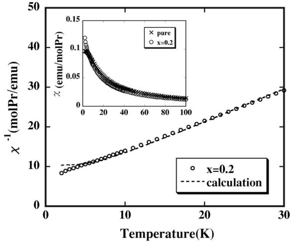
FIG. 1. Temperature dependence of the inverse susceptibility for  $x=0.2$ . The broken curve shows the calculated result based on the CEF level scheme; the ground state is  $\Gamma_3$  and the first excited one is  $\Gamma_4$ , with an energy splitting of 19 K. The next excited state is  $\Gamma_5$ , with an energy splitting of 46 K from the ground state. Inset: temperature dependence of the susceptibility for  $x=0$  and  $x=0.2$ .
