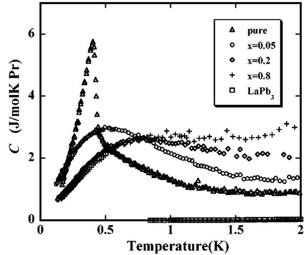
FIG. 2. Temperature dependence of the specific heat for pure and mixed systems with  $x=0.05$ ,  $0.2$ , and  $0.8$ , where the specific heat is normalized by the Pr atomic concentration. The reference compound  $\text{LaPb}_3$  is also shown.
