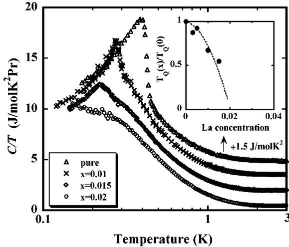
FIG. 3.  $C/T$  plotted on a logarithmic temperature scale for pure  $x=0.01$ ,  $0.015$ , and  $0.02$  cases. The data of the pure,  $0.01$  and  $0.015$  cases are shifted by  $1.5$  ( $\text{J/mol K}^2 \text{ Pr}$ ). The sharp peak due to the quadrupolar ordering is shifted to the lower temperatures with an increase of the La concentrations. Inset: the concentration dependence of  $T_Q(x)/T_Q(0)$ . The dotted line is a guide to the eye.
