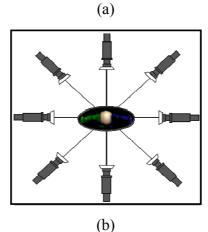
Fig. 5.10 (a) Eight views of an actor performing a motion, (b) surrounding camera concept.
