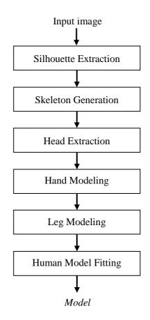
Fig. 4.5 System framework for motion modeling
