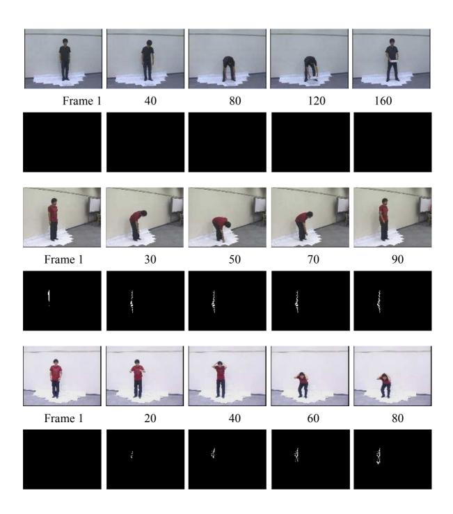
Fig. 2.4 Examples of different actions and corresponding XOR images; top row contains key frames and bottom row is cumulative motion images starting form frame 1. Top to bottom: Carry (frontal view), Pickup (Right view), and Headache-and-Sit (Left view).
