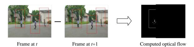
Fig. 7.8 Optical flow computation from L-K tracker output.
