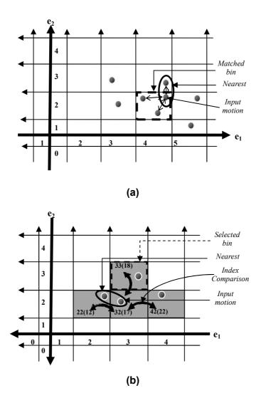
Fig. 5.5 Occurrence of the *boundary problem*: (a) Point inside the oval is the nearest; but other point will be selected, (b) Index comparison of input (32) with other three 22, 33 and 42. The point inside 22 is the nearest but 33 is selected.
