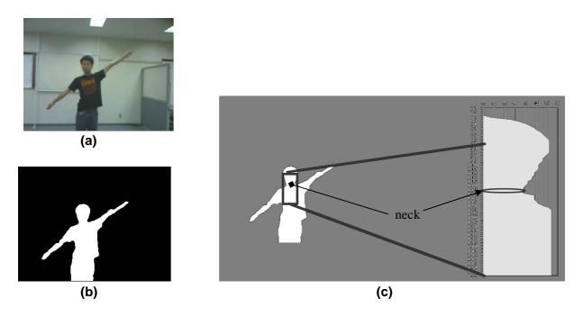
Fig. 4.9 Neck positioning. (a) original frame, (b) silhouette image, (c) neck positioning by vertical histogramming
