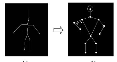
(a) (b) Fig. 4.10 Hand modeling for a frontal view. (a) a hand skeleton, (b) hand modeling
