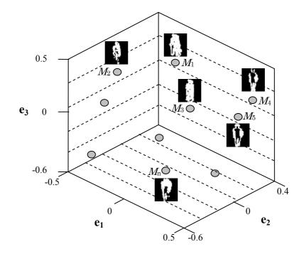
Fig. 3.2 An example of an eigenspace and projected motion images  $(M_1, M_2, ..., M_n)$ . MHI motion representations are used for the illustration. Each motion is represented as a single point within the space. Three major dimensions of the eigenspace are displayed.
