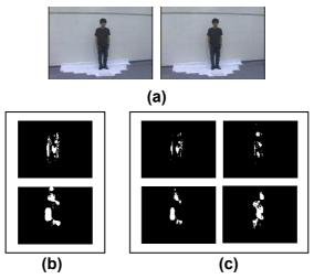
Fig. 6.3 Computation of an optical flow image. (a) Original consecutive frames, (b) Intensity image for the horizontal(x) and vertical(y) components of the optical flow generated from original consecutive frames, (c) Intensity image of four separate channels of x and y. top row:  $x^+$ ,  $x^-$ , bottom row:  $y^+$ ,  $y^-$ .
