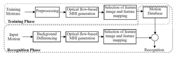
Fig. 6.10 System framework for the cluttered outdoor recognition
