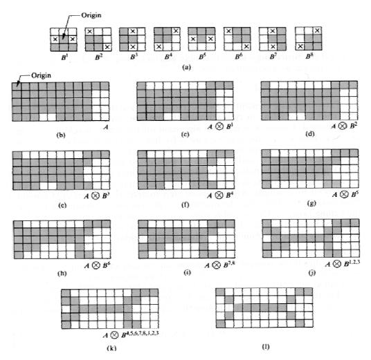
Fig. 4.6 An example of the implementation of the *thinning algorithm* on an image A.
