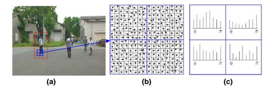
Fig.7.6 Histograms of oriented gradients: (a) A 64×128 search window (a rectangle enclosing the leftmost person), (b) a 16×16 block of 4 cells, (c) the histograms of oriented gradients corresponding to the 4 cells.
