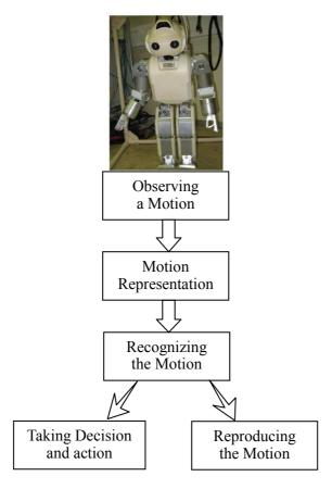
Fig. 1.1 Basic tasks within an intelligent robot system
