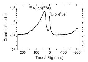
FIG. 2. TOF spectrum for  $^{197}$ Au taken by the NaI(Tl) detector at  $E_n = 531$  keV. The peak at 0 ns is from the  $^7$ Li(p,  $\gamma$ ) $^8$ Be reaction and the broad peak is due to the  $\gamma$  ray from the keV neutron capture reaction by  $^{197}$ Au.
