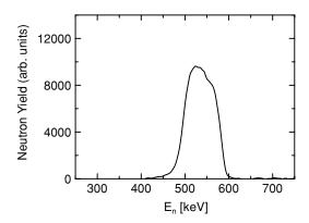
FIG. 1. Neutron energy spectrum taken by a  $^6\mathrm{Li}$  glass scintillation detector with a TOF method.
