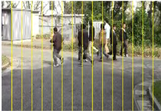
Fig. 2.6 An image frame and its division into blocks
