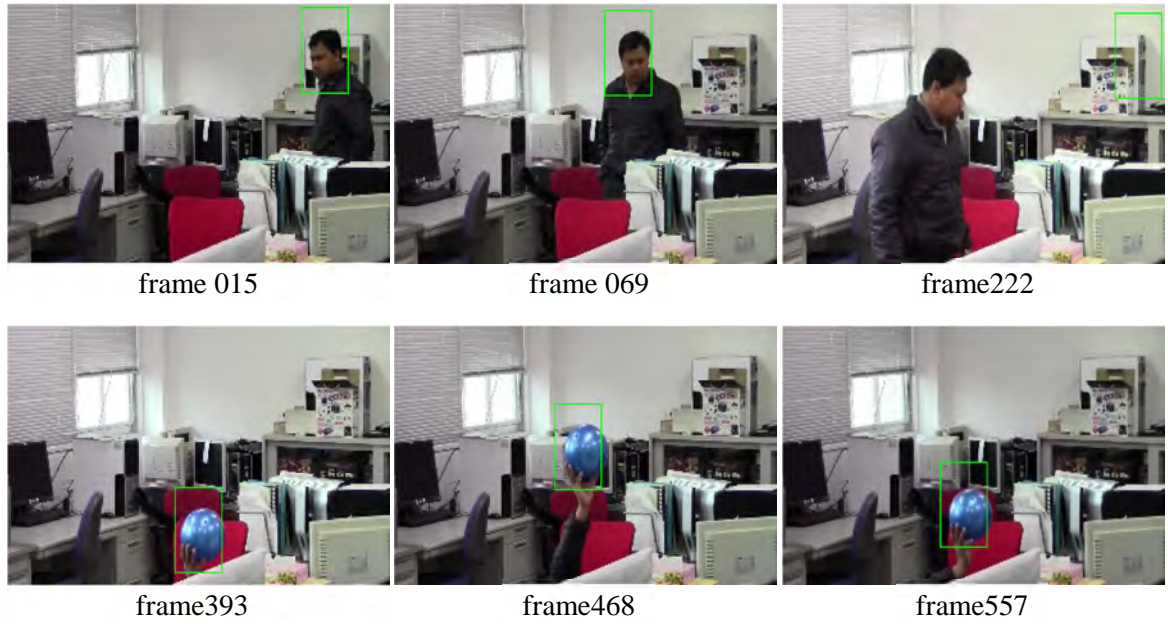
Fig. 5.3 The results of head motion detection using the comparative method 3-1.
