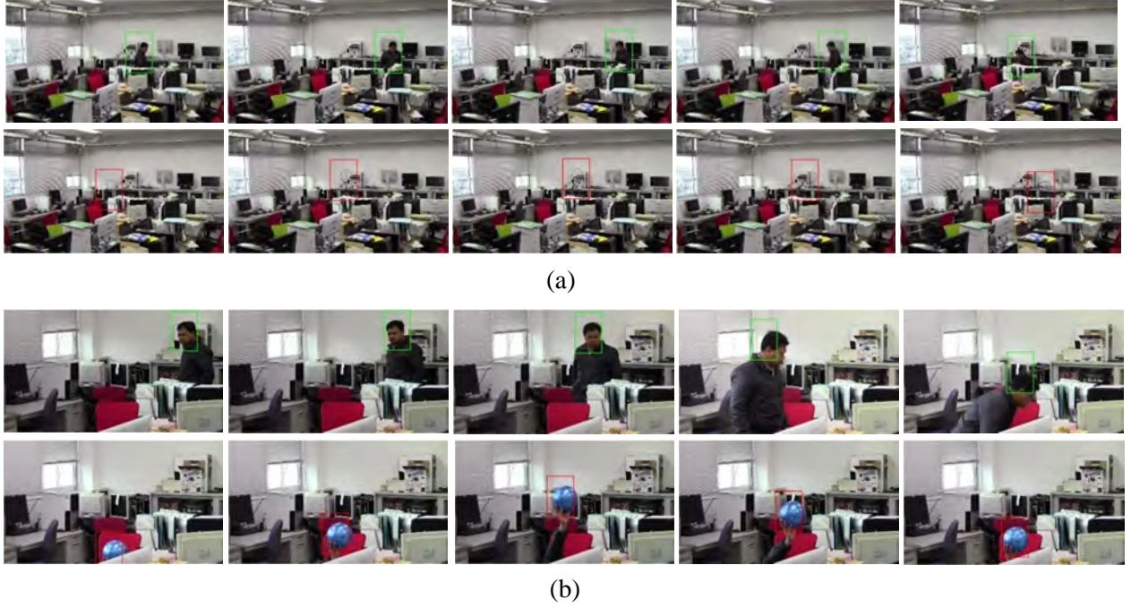
Fig. 4.12. Performance of head detection. The green box shows that the proposed system detects a motion and a head, the red box shows that the system detects a motion but not a head . (a) Video 1: The system can distinguish a head and a racket. (b) Video 2: The system can distinguish a head and a ball
