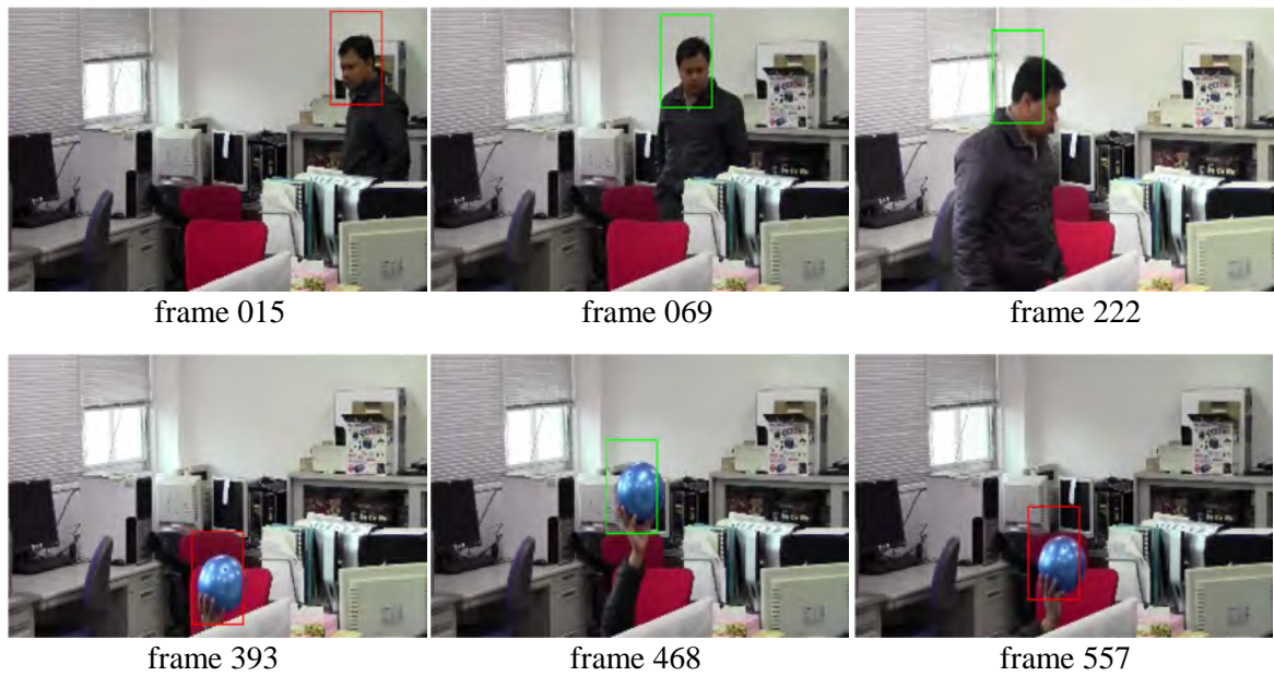
Fig. 5.4 The results of head motion detection using the comparative method 3-2.
