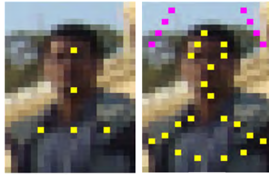
(a) (b) Fig. 4.10 The coordinate of reference pixel: (a) The distance function method, (b) LNP method: yellow are foreground, magenta are background.
