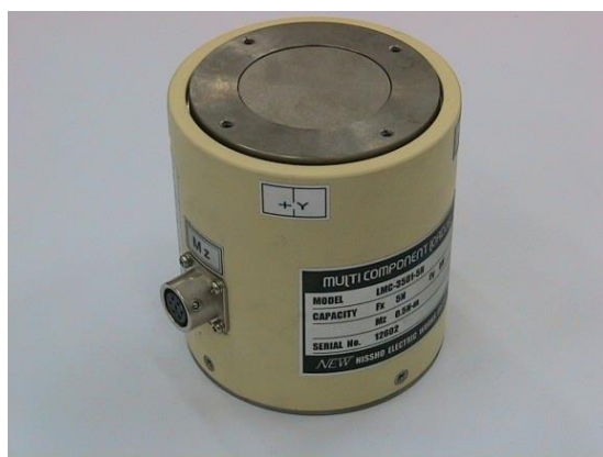
Fig. 3.3.4 Three-component Force Balance LMC-3501-5N
