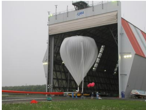
Fig. 1.1.8 Highest Altitude Balloon Using The Ultra-thin Polyethylene Film (Copyright ©ISAS/JAXA)
