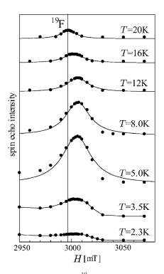
FIG. 2. Profile of field-swept <sup>19</sup>F NMR spectra for 120 MHz at different temperatures. The solid line indicates the free <sup>19</sup>F resonance field for 120 MHz.
