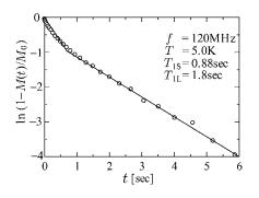
FIG. 3. A recovery of the intensity of a spin echo signal of <sup>19</sup>F for 120 MHz at T=5.0 K. The solid line shows a two-exponential expression with  $T_{1S}$ =0.88 sec and  $T_{1L}$ =1.8 sec.
