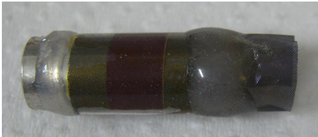
Final cell after injecting the electrolyte and sealing with UV-resin.
